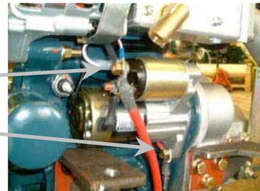
**Note:** The two way plug on panel loom will only have a corresponding socket to connect into from the engine if a 2<sup>nd</sup> alternator is fitted which requires this connection. Engines with only one alternator do not utilise this connection.
