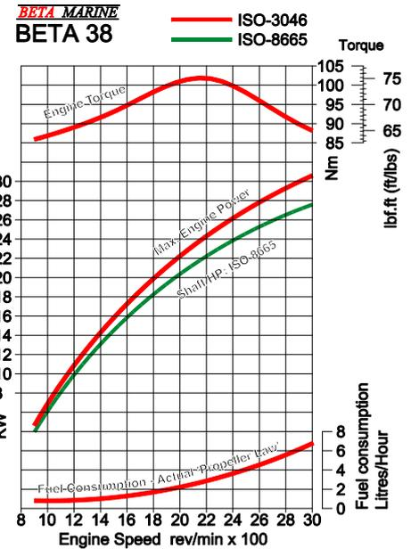
Fuel Consumption based on theoretical propeller loading - matched at full speed
